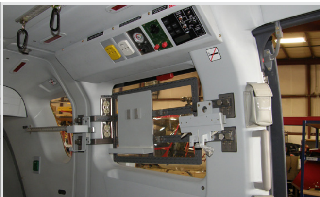
Medical Equipment Rack
